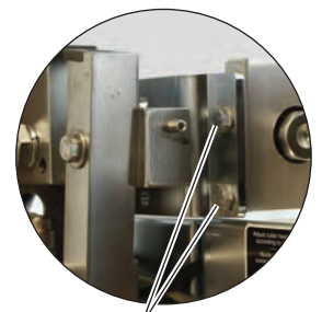
Hexagonal head screws 2 x M6 x 12 mm
